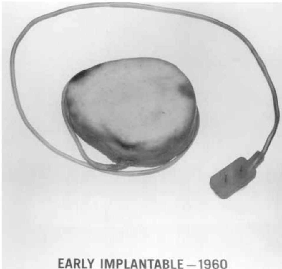
*Figure 10. The Chardack-Great batch implantable pacemaker, 1960, which Medtronic obtained the rights to produce. The pulse generator is encapsulated in silicone rubber and is fitted with a Hunter-Roth platform electrode. Courtesy of Medtronic, Inc.*
